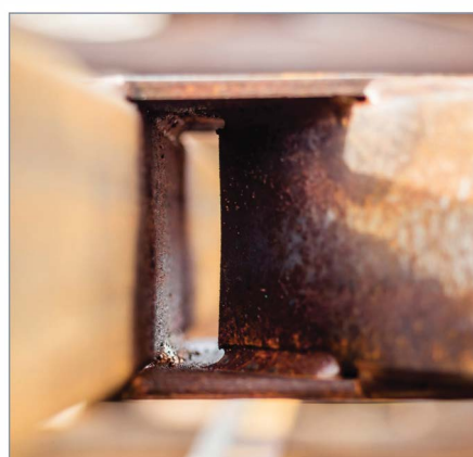
ZINC FREE FLOW. Stopping short cross beams eliminates air locks and allows free flow of zinc through the fabrication.
