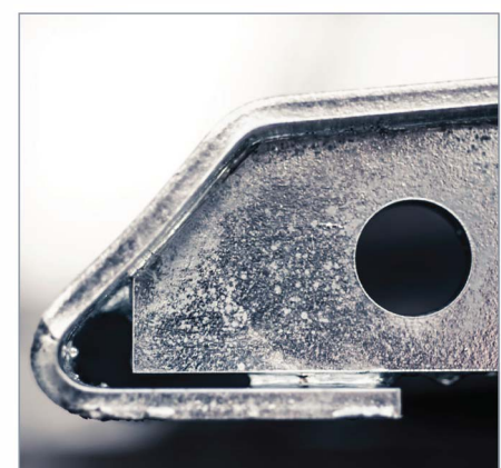
AIR LOCK PREVENTION. The photo shows how stopping short the end plate prevents an air lock.
