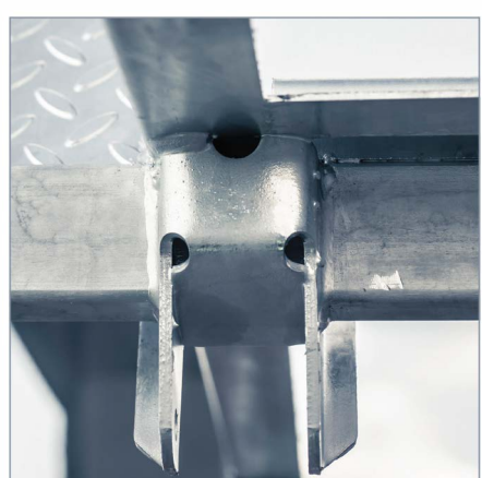
HOLE STAMPING. Holes stamped out prior to weld assembly.
